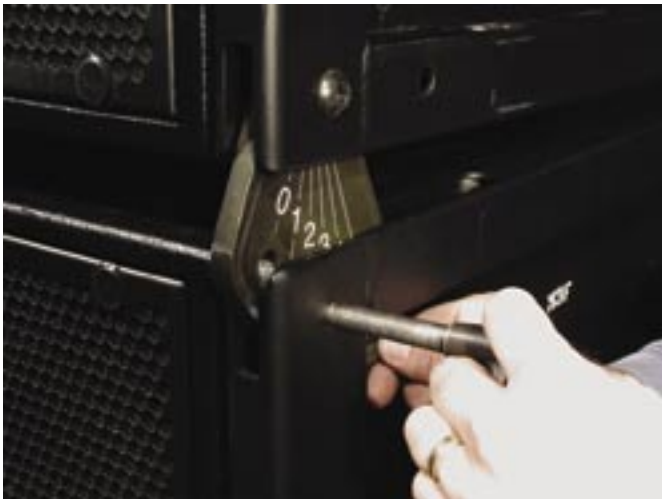
Figure 28. Inserting QRP at 3°
